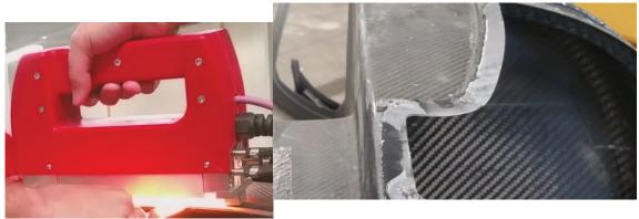
Split glued layers of non-homogeneous materials, without damaging the single layers.
