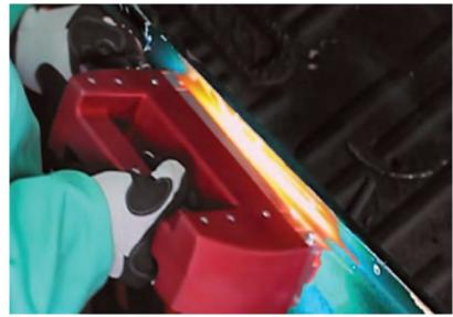
The heating tool of the 3546 is provided with a no-contact temperature sensor, which allows modulating the power of the heating tool to keep the temperature constant.
